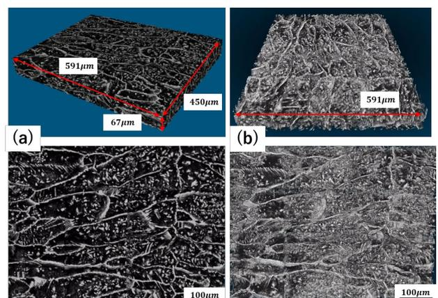
**Fig. 3** (a): The three dimensional model of welds rebuild by serial sectioning method, (b): The three dimensional model of welds only retains the austenite phase.
