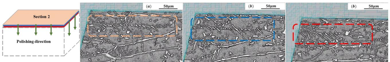
Fig. 6 Observation results of the same Widmanstätten austenite at different depths of section 2.
