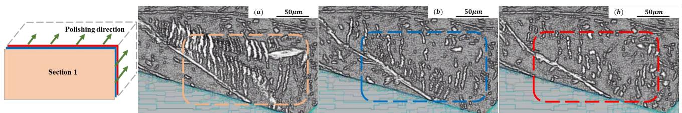
Fig. 5 Observation results of the same Widmanstätten austenite at different depths of section 1.
