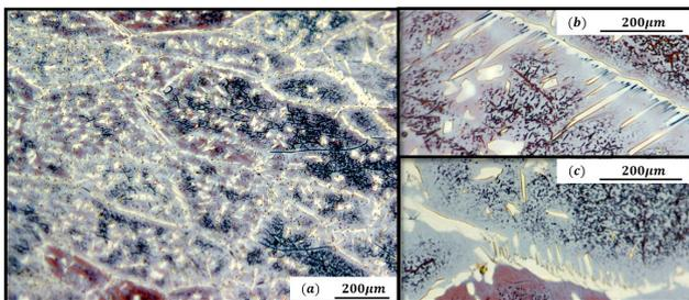
**Fig. 1** (a):Microstructures in laser welds of duplex stainless steel (S32101), (b)(c): Widmanstätten austenite at grain boundaries.
