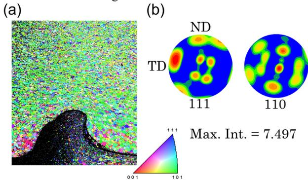
Fig. 8 IPF map around the small anchor taken from the LD direction and pole figure.
