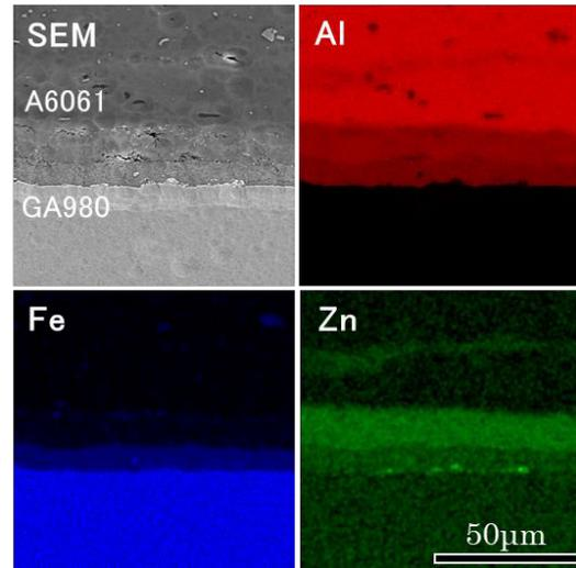
**Fig. 4** Chemical mapping around the interface produced under the pin.
