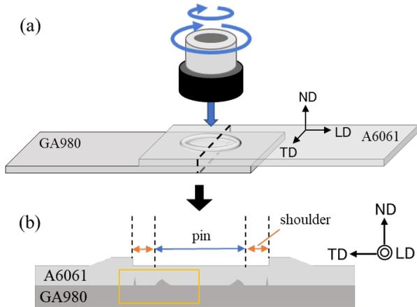
**Fig. 1** Schematic of (a) Sc-RFSSW process and (b) cross-section of the bonded specimen.
