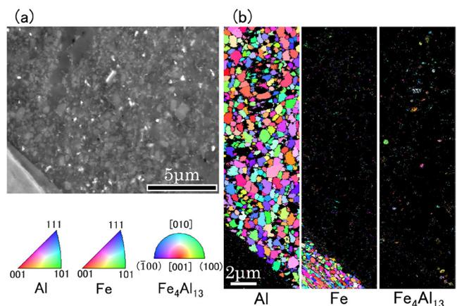
**Fig. 7** (a) SEM image of the small particles in the rolled-up region denoted by yellow arrows in Fig. 6 and (b) IPF map.
