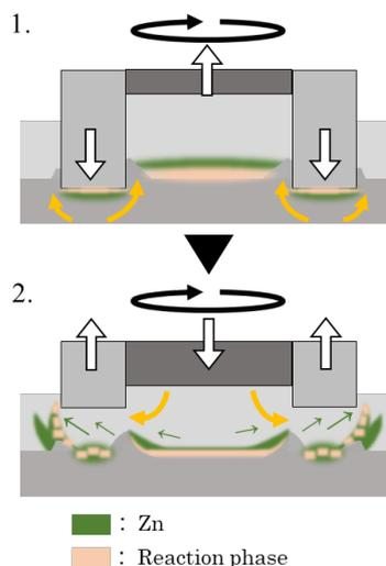
Fig. 9 Schematic of the welding process of Sc-RFSSW.
