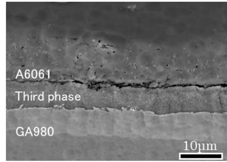
**Fig. 3** SEM image of the interface produced under the pin.
