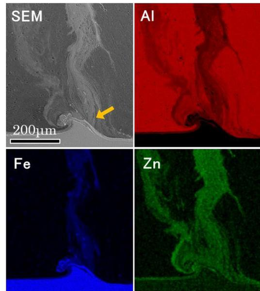
**Fig. 6** Chemical mapping around the small anchor.
