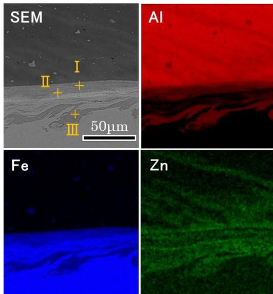
**Fig. 5** Chemical mapping around the interface produced under the shoulder.
