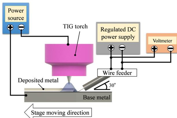
Fig. 3 Schematic illustration of the experimental setup for milli-scale WAAM
