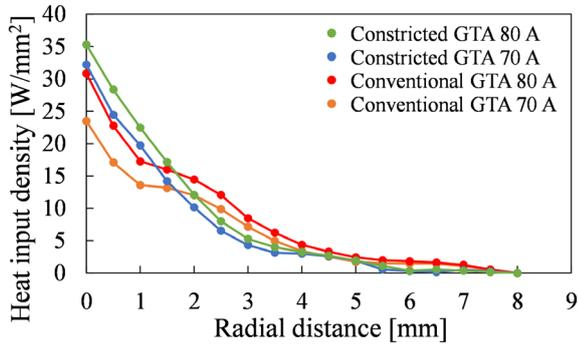
Fig. 8 Heat input density distribution on the anode surface for each arc current and heat source
