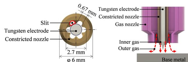
(a) Cross-section of the constricted nozzle (b) Internal structure of the constricted GTA torch
