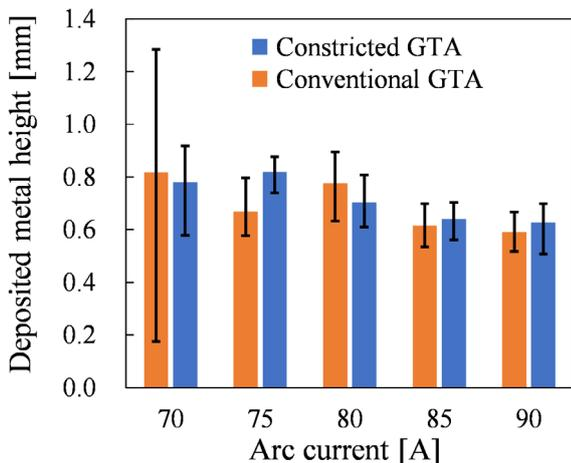
Fig. 4 Measurement results for deposited metal height for each current and heat source
