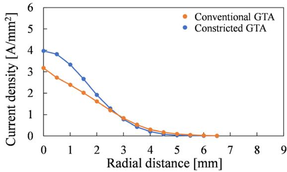
Fig. 6 Current density distribution on the anode surface at an arc current of 70 A for each heat source
