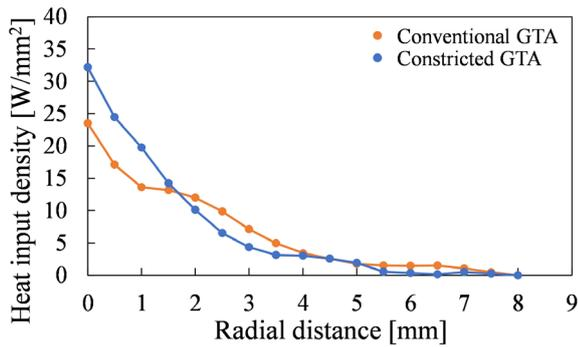
Fig. 7 Heat input density distribution on the anode surface at an arc current of 70 A for each heat source
