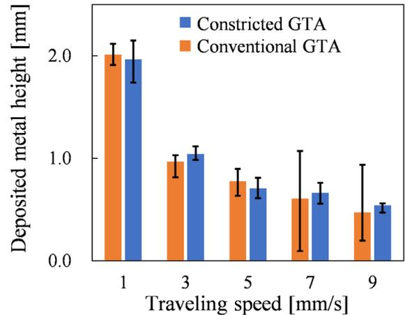
Fig. 5 Measurement results for deposited metal height for each traveling speed and heat source
